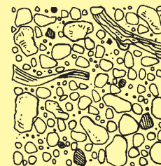
Poorly graded and round sand with organic debris.
